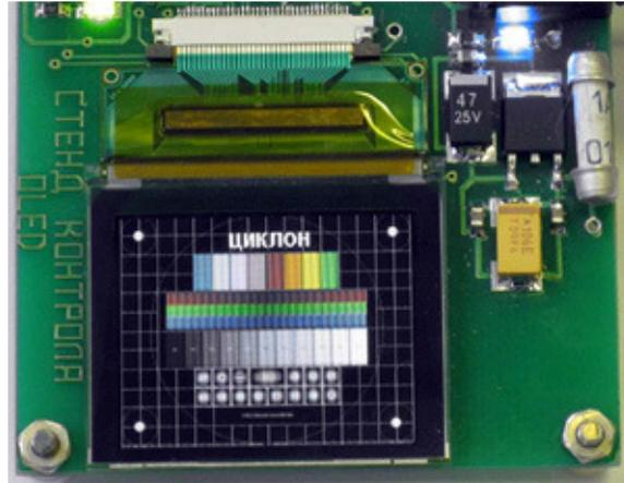
Since resistance to external influences is a significant parameter for organic LED devices, the displays were subjected to mechanical, climatic, and thermal tests. They reliably operate from  $-20$  to  $+55$  °C, under single impacts up to 150 g, and exposed to vibration within the 10-55 Hz range with multiple impacts up to 10 g.
