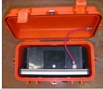
Tests compared this new instrument with three other similar devices. The radar successfully coped with all the tasks and was able to detect people under four different objects, including underground shelters and multi-meter concrete block piles. The device emits radio waves that detect any human movements, even slight thorax vibrations from breathing.
