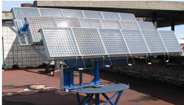
The solar battery modules developed by PTI scientists are composed of the photoconverters being placed on heat-removing substrates at the focus distance from mini-lenses. The mini-lenses provide for a thousandfold solar radiation concentration. This technology reduces both the solar batteries' active surface area and their cost.
